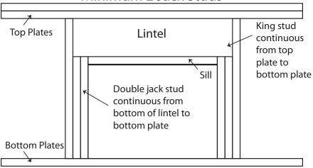
These spans are generated using Manitoba Building Code span Tables and cwc 2004 span tables forming part of MBC 9.23, with an assumed snow load of 2.0 kpa and 4/12 roof slope. The lintel tables below indicate size of openings and acceptable lintel spans. For additional sizes and spans, please refer to the Manitoba Building Code span tables.
